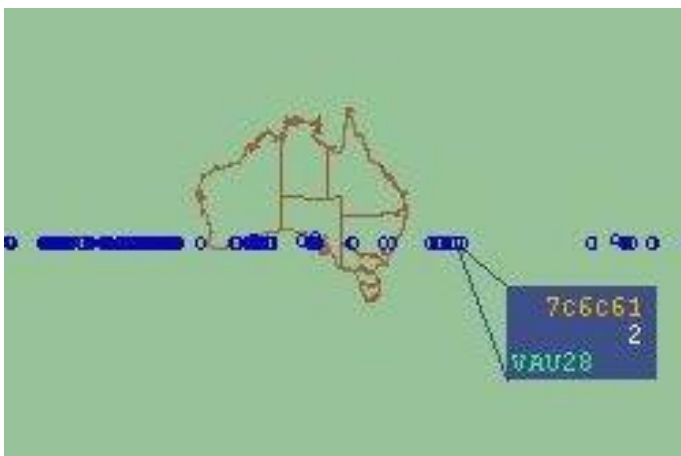
Figure 1 - Track Jumping problem with TPR901
